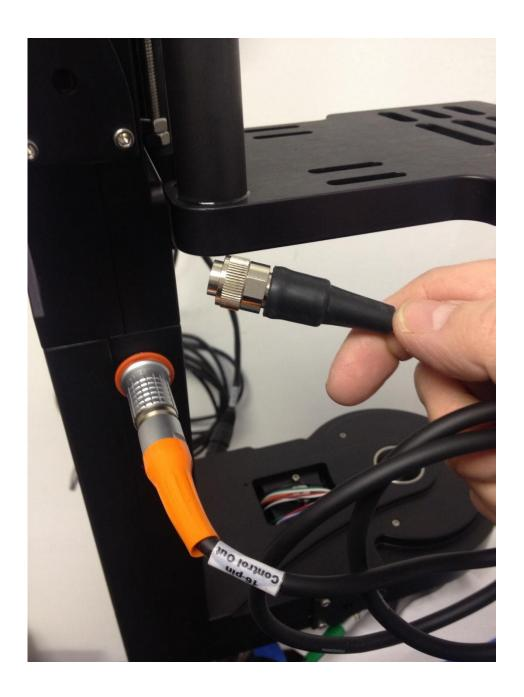
VZCP-C09 (\$399 each) – Lens control cable. MUST be optional, because there are MANY different types of connectors and software prototcols. Head outputs lens control via 16pin 2B Lemo. Customer must specify connector type and lens model at time of order.
