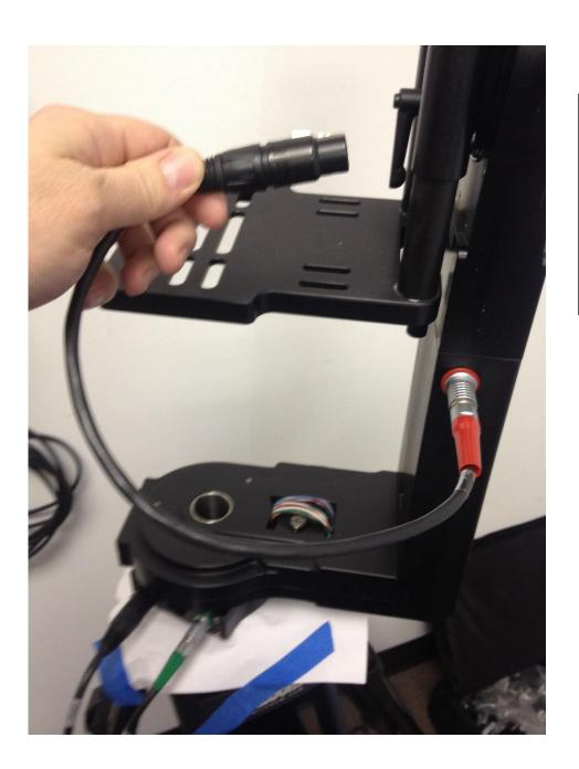
VZCP-C10 power cable is shown with 4pin XLR option. Connector/pinouts for camera power cable must be specified at time of order.
