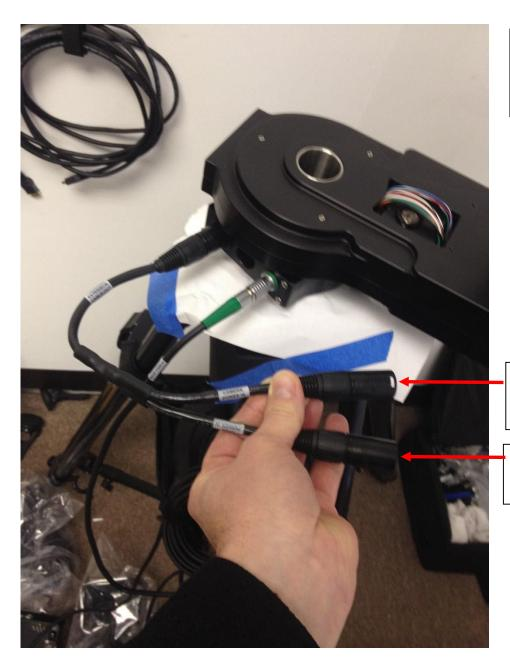
Note: CinemaPro-Jr DOES NOT supply power to any camera. Camera power must be supplied by the end user. Our camera power cable option is ONLY a pass-thru to streamline cabling and avoid cable twisting.
